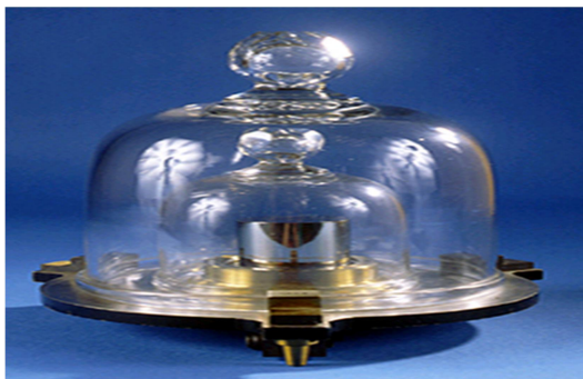
Figure 1.13: This replica prototype kilogram as previously defined is housed at the National Institute of Standards and Technology (NIST) in Maryland.
